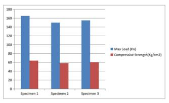
Figure 1: Graph Showing Compressive Strength for 1:2 Plastic to Sand Ratio
