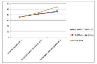
Figure 6: Graphical representation of Increase in Temperature of Plastic Bricks and Clay Bricks
