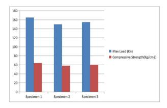
Figure 3: Graph Showing Compressive Strength for 1:4 Plastic to Sand Ratio
