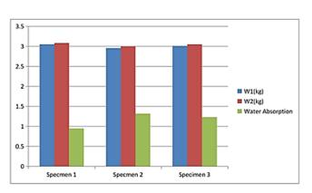
Figure 4: Graph Showing Water Absorption Test for 1:2 Ratios Plastic to Sand Bricks
