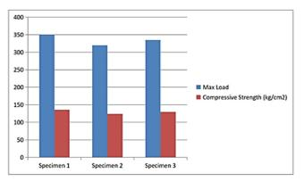
Figure 2: Graph Showing Compressive Strength for 1:3 Plastic to Sand Ratio
